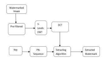
fig 2.3 Extraction Block diagram
