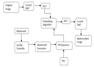
fig 2.2 Embedding Block Diagram
